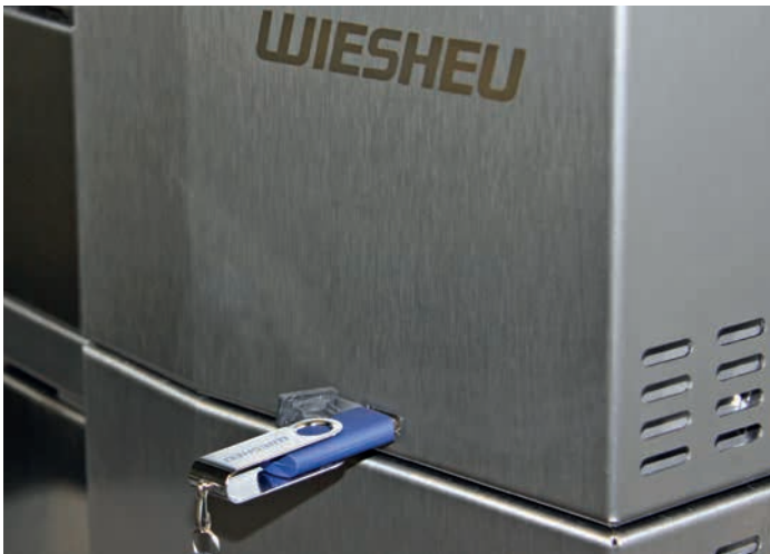
Programming of control unit via USB port
